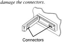
To minimize this possibility, periodically wipe the connectors with a cotton swab or cloth moistened with alcohol, being careful not to
